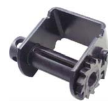
PP3025 4" Standard Slider Winch Working Load Limit: 5,500 lbs. Breaking Strength: 16,500 lbs. Weight: 9.1 lbs./4.12kgs.
