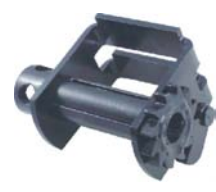
PP3054 4" Low Profile Double L Track Winch Working Load Limit: 5,500 lbs. Breaking Strength: 16,500 lbs. Weight: 7.9 lbs./3.6 kgs.
