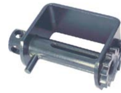
PP3049 4" Standard Weld-on Combination Winch Working Load Limit: 5,500 lbs./Webbing 3,335 lbs./Cable Breaking Strength: 16,500 lbs./Webbing 10,000 lbs./Cable Weight: 10.6 lbs./4.8 kgs.
