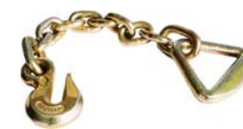
PP5002 18" Chain Anchor w/3" Forged Delta Ring, Yellow Dichromate Zinc Plating WLL: 5,400 lbs. Weight: 3.6 lbs./1.63 kgs.
