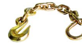
PP5001 18" Chain Anchor w/Pear Link, Yellow Dichromate Zinc Plating WLL: 5,400 lbs. Weight: 2.92 lbs./1.33 kgs.
