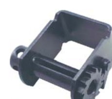
PP3026 4" High Profile Slider Winch Working Load Limit: 5,500 lbs. Breaking Strength: 16,500 lbs. Weight: 9.7 lbs./4.4 kgs.
