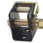
PP3003 2" Lashing Winch w/Hex Head On Right Working Load Limit: 3,333 lbs. Breaking Strength: 10,000 lbs. Weight: 3.4 lbs./1.55 kgs.
