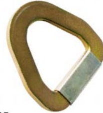
PP2165 2" HD Stamped Delta Ring w/Steel Wear Pad WLL: 3,600 lbs. Weight: 0.33 lbs./0.15 kgs.
