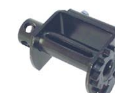
PP3012 4" Low Profile Portable Winch w/ 2 set screws Working Load Limit: 5,500 lbs. Breaking Strength: 16,500 lbs. Weight: 9.6 lbs./4.36 kgs.
