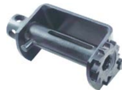
PP3048 4" Low profile Weld-on Combination Winch Working Load Limit: 5,500 lbs./Webbing 3,335 lbs./Cable Breaking Strength: 16,500 lbs./Webbing 10,000 lbs./Cable Weight: 9.7 lbs./4.4 kgs.
