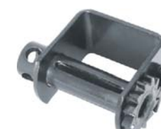
PP3009 4" Standard Weld-on Winch Working Load Limit: 5,500 lbs. Breaking Strength: 16,500 lbs. Weight: 8.7 lbs./3.96kgs.
