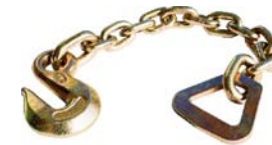
PP5003 18" Chain Anchor w/2" Delta Ring, Yellow Dichromate Zinc Plating WLL: 3,335 lbs. Weight: 2.3 lbs./1.05 kgs.
