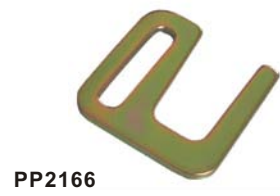
PP2166 2" Slat Hook WLL: 1,000 lbs. Weight: 0.21 lbs./0.095kgs.
