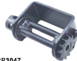
PP3047 4" Standard Weld-on 3-Bar Winch Working Load Limit: 5,500 lbs. Breaking Strength: 16,500 lbs. Weight: 13.2 lbs./5.98 kgs.
