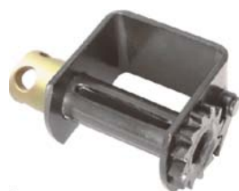
PP3309 4" Ratchet Cap Standard Weld-On Winch Working Load Limit: 5,500 lbs. Breaking Strength: 16,500 lbs. Weight: 9.9 lbs./4.52kgs.
