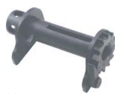
PP3032 4" Weld-on 2-pc Leg Bracket Combination Winch Working Load Limit: 5,500 lbs./Webbing 3,335 lbs./Cable Breaking Strength: 16,500 lbs./Webbing 10,000 lbs./Cable Weight: 6.8 lbs./3.1 kgs.
