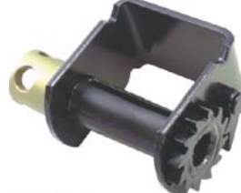
PP3325 4" Ratchet Cap Slider Winch Working Load Limit: 5,500 lbs. Breaking Strength: 16,500 lbs. Weight: 10.3 lbs./4.68kgs.
