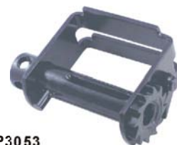
PP3053 4" Combination Double LTrack Winch Working Load Limit: 5,000 lbs./Webbing 3,335 lbs./Cable Breaking Strength: 15,000 lbs./Webbing 10,000 lbs./Cable Weight: 9.9 lbs./4.5 kgs.
