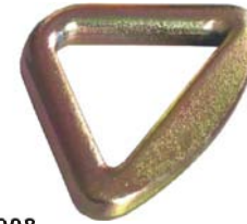
PP5008 3" HD Forged Delta Ring WLL: 6,000 lbs. Weight: 0.88 lbs./0.4 kgs.
