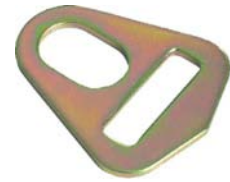
PP2170 2" Flat Delta Ring WLL: 5,400 lbs. Weight: 0.28 lbs./0.13 kgs
