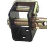
PP3004 2" Lashing Winch w/Round Head Working Load Limit: 3,333 lbs. Breaking Strength: 10,000 lbs. Weight: 3.4 lbs./1.55 kgs.
