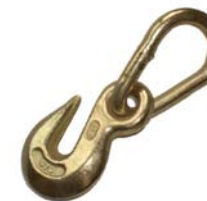
PP5004 3/8" Grab Hook w/Pear Link, Yellow Dichromate Zinc Plating WLL: 5,400 lbs. Weight: 1.32 lbs./0.6 kgs.
