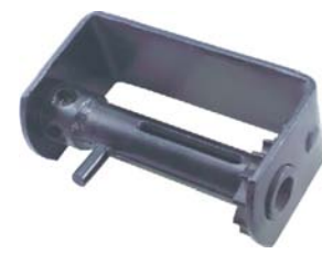
PP3050 4" Weld-on Combination Box Winch Working Load Limit: 5,500 lbs./Webbing 3,335 lbs./Cable Breaking Strength: 16,500 lbs./Webbing 10,000 lbs./Cable Weight: 11.9 lbs./5.4 kgs.
