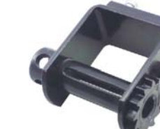
PP3014 4" High Profile Portable Winch w/ 2 set screws Working Load Limit: 5,500 lbs. Breaking Strength: 16,500 lbs. Weight: 9.6 lbs./4.36 kgs.
