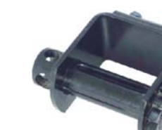
PP3013 4" Standard Portable Winch w/ 2 set screws Working Load Limit: 5,500 lbs. Breaking Strength: 16,500 lbs. Weight: 9.2 lbs./4.20 kgs.
