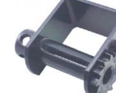
PP3011 4" Storable Weld-on Winch Working Load Limit: 5,500 lbs. Breaking Strength: 16,500 lbs. Weight: 8.8 lbs./4.4kgs.
